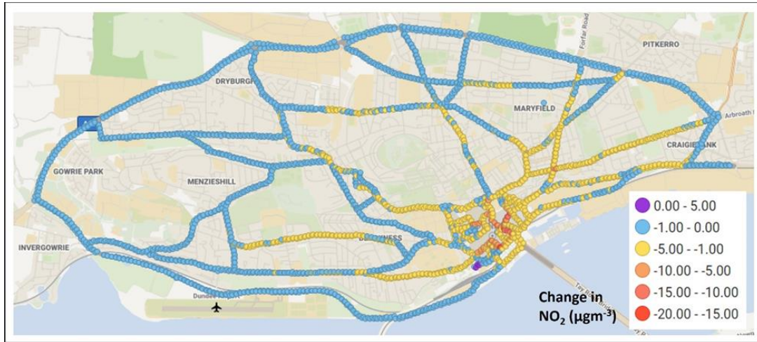
Figure 2.5 Relative changes in NO 2 concentration between Reference and LEZ cases across the entire model domain
