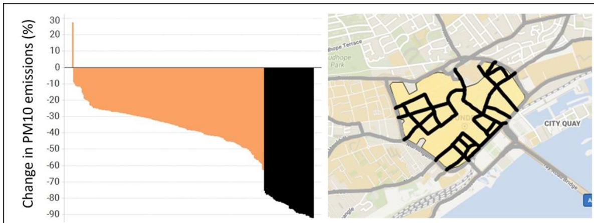
Figure 2.6 Ranked changes in PM 10 emissions (%) on all roads (The greatest reductions occur inside the LEZ as highlighted in black)
