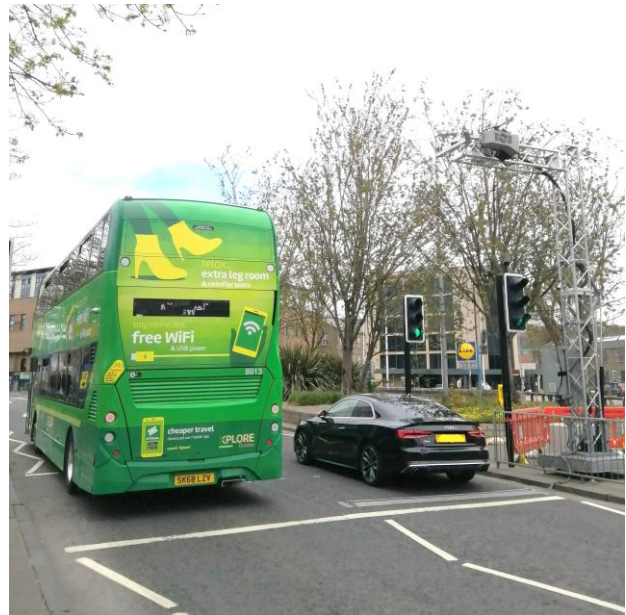
Figure 3 Illustration of how EDAR unit measures exhaust emissions from on-road vehicles (left) and an EDAR system measuring emissions from a vehicle in Dundee (right)
